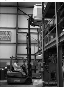
A container of material goes up to second floor level to begin its descent through the blending process to ground level.
